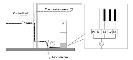
Heater's electrical connection, double input
