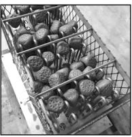
7. Insert the top part element guides so that they lean against the horizontal steel pillars. Place appx. 25-40pcs small KERKES ceramic stones between the elements depending on the model. That way we can avoid the elements to bend against each other.
