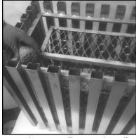
9. Set the stones (large and small Kerkes tetra stones) between the inner and outer frame. At last set the stones on top of the inner frame and the coverpart/lid.
